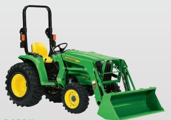
**3032E with D160 Loader** 31.1HP / 4WD / Yanmar 3 Cylinder Diesel Engine / Dual Hydraulic Pumps
